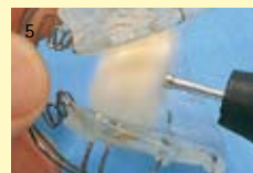
The cotton buff allows polishing at spots of the ortho-dontic appliance which can not be reached with the polishing motor. Extremely soft cotton threads produce a mirror-like high luster.
