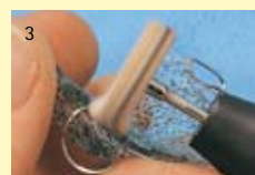
The three-layer felt buff polishes clasp transitions gently and quickly.
